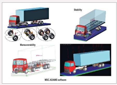
Fig. 2. Virtual testing of a medium-duty articulated road-train
