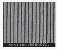
Nanoporous aluminum oxide is used for creating new light-emitting structures (the Belarusian State University of Informatics and Radioelectronics)
