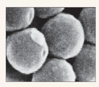
Self-assembly of dielectric nanoparticles into a structure of a "photonic crystal" type (B.I. Stepanov Institute of Physics jointly with the Institute of Powder Metallurgy)
