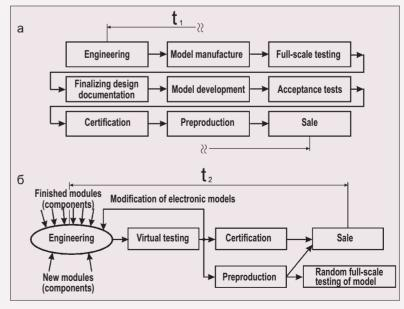
Fig. 1. Approaches to developing new equipment: a — conventional; b — innovative
