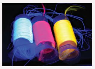
Mogilevkhimvolokno OJSC-produced fiber dyed with the ICNM-developed fluorescent dyes (UV light)
