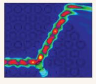
Planar photonic crystal waveguide: geometrical construction (on the left) and calculated intensity of electromagnetic field (on the right). Calculations by A.V. Lavrinenko (BSU)
