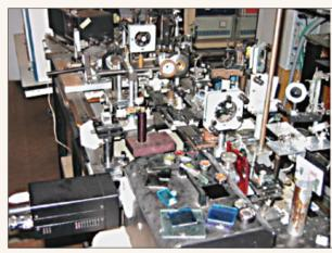
The model of the femtosecond SRS-amplifier on a Raman-active crystal
